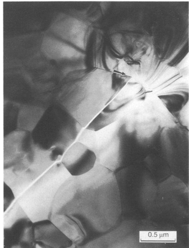
Figure 3 Near-tip region in composite B observed by TEM. The crack tip is arrowed.
