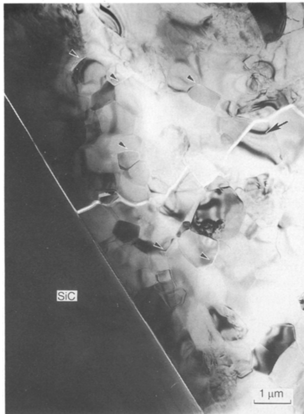
Figure 1 Typical crack path observed by TEM in composite A with a high percentage of intergranular fracture in the \text{Si}_3\text{N}_4 matrix and debonding at the carbide interface. The crack propagation direction is arrowed. Small arrows indicate microcracking.
